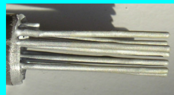
Coating appeared intact after 14-day exposure
