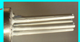
Signal was significant even though coating appeared intact after 14-day exposure
