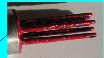
A small area of coating peeled off after 7-day exposure
