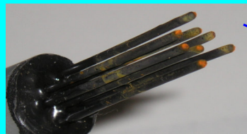
Rust observed on all defected areas after 7-day exposure
