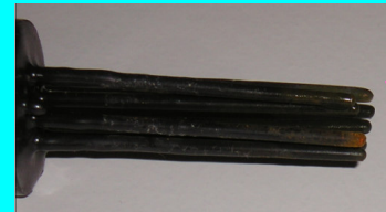
Rust observed on defected areas after 7-day exposure
