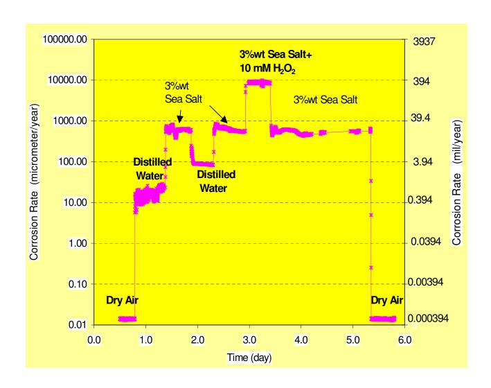
Typical Responses of Carbon steel Multielectrode Sensors to the Changes of solution chemistry.
