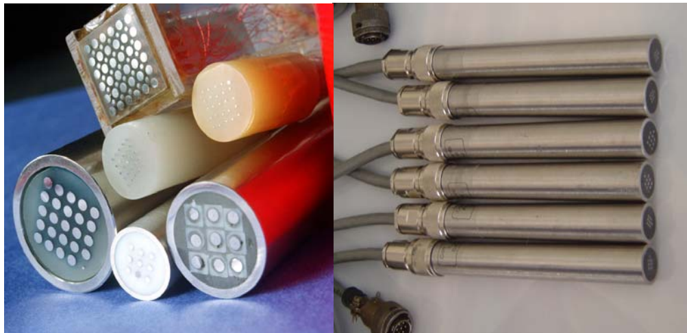
Figure 9. Typical coupled multi-electrode sensor probes for applications in corrosion monitoring and electrochemical studies. Source: Ref. 75 and Ref. 93.
