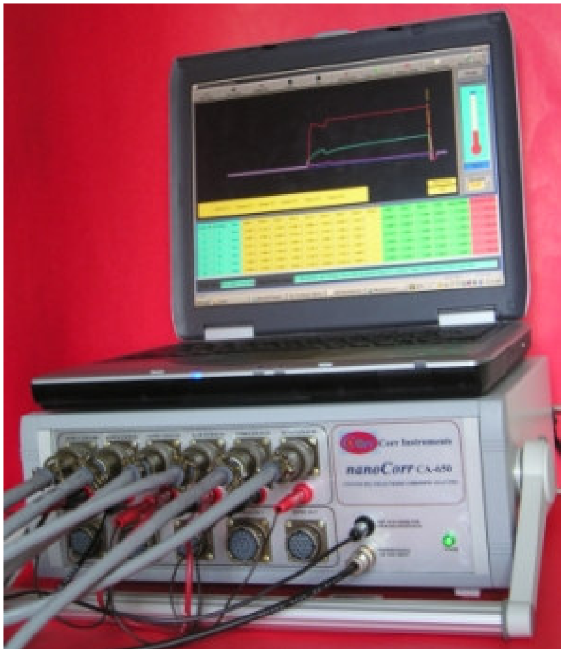
Figure 2. Experiment setup: Six sensors connected to the coupled multielectrode corrosion analyzer system.
